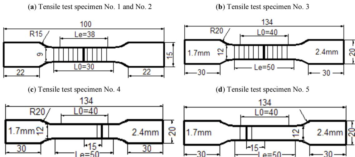
**Fig. (2).** Profile and dimensions of tensile test specimens 67089.
