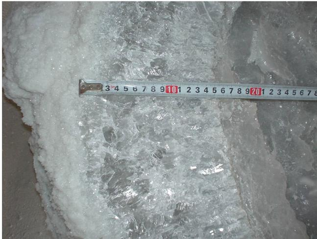
**Fig. (12).** Photograph of the large MgO single crystal grown using adaptive neuro-fuzzy inference system.
