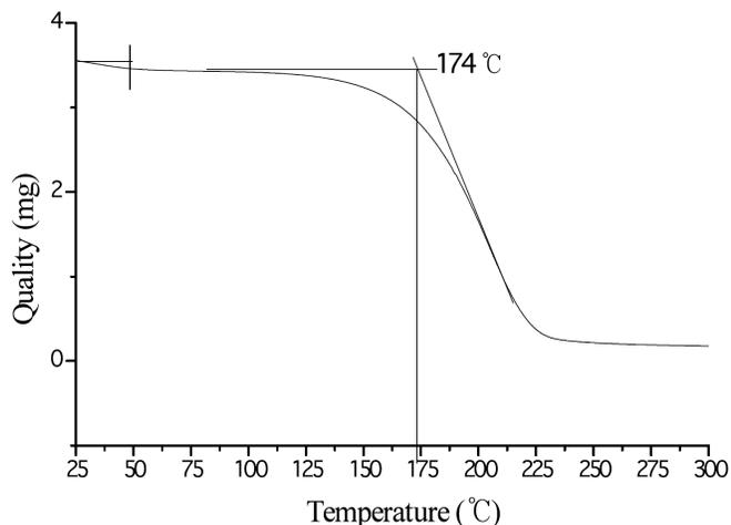
Fig. (4). TGA curve of the LCA.
