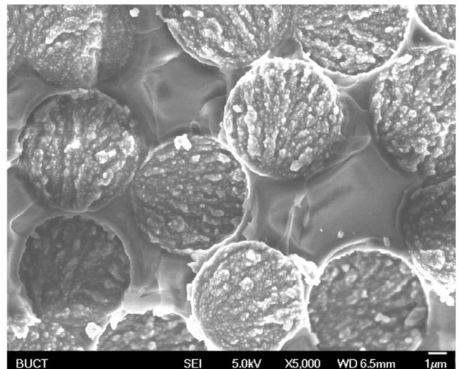
Fig. (7). SEM images of sized high modulus carbon fiber and epoxy resin composites.
