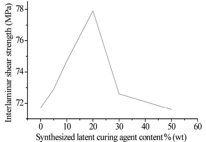
Fig. (6). Interlaminar shear strength of composites.
