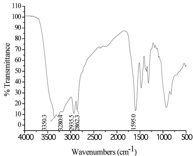
Fig. (2). FTIR spectrum of ethylenediamine.
