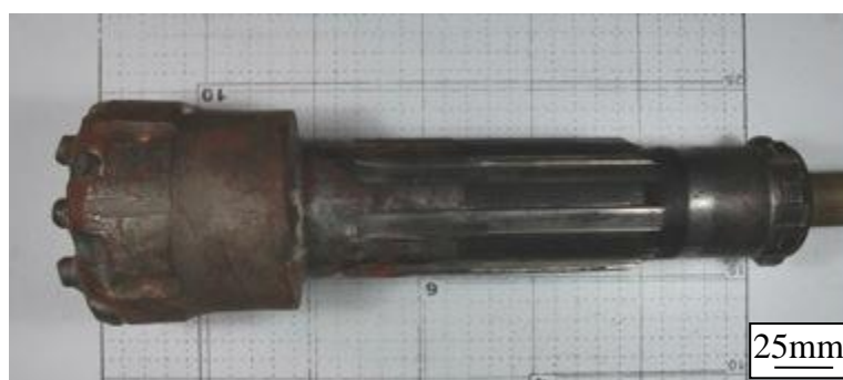
Fig. (2). The qualified drill bit scrapped after serving for a long time.
