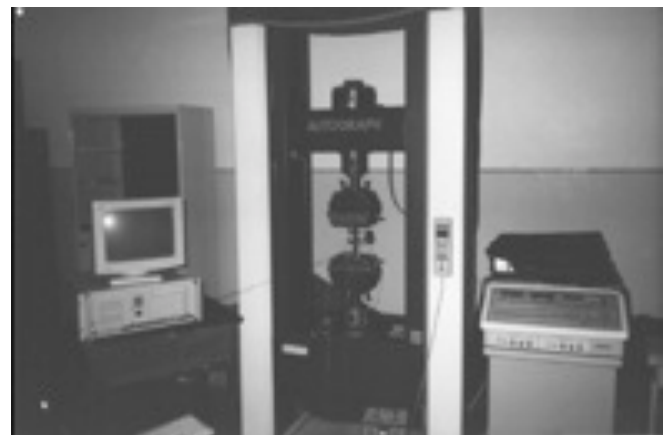
Fig. (3). AG250KN universal material experiment machine.
