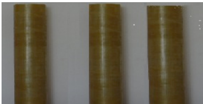
Fig. (2). Multi-directional filament winding material tubes.
