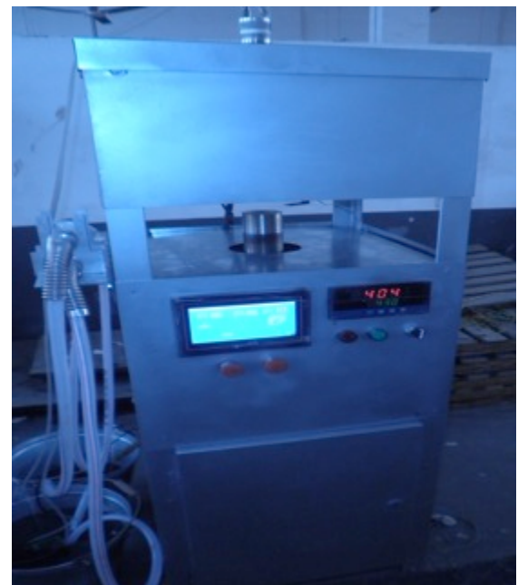
Fig. (3). Experimental setup for glass compression tests (a) schematic diagram (b) GMP setup.
