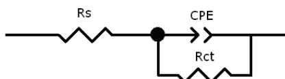
Fig. (2). Equivalent electrical circuit of the interface of mild steel / HCl solution both in the absence and presence of CBE or CBEK.
