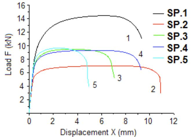
**Fig. (4).** Displacement and load curve of tensile testing specimens.
