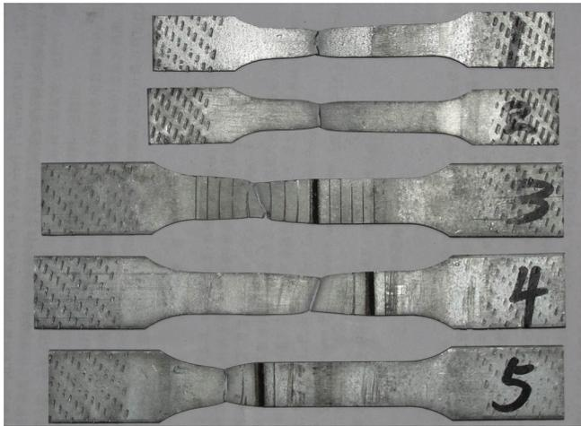
**Fig. (5).** The results of specimens after tensile test.
