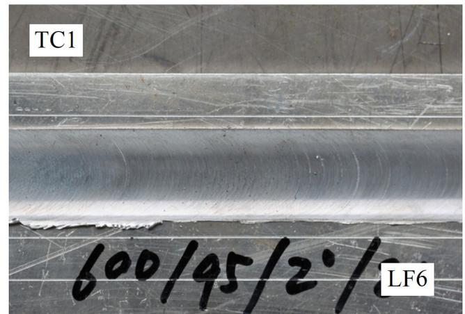
Fig. (7). Surface morphology of of Ti/Al dissimilar alloys lap joint.
