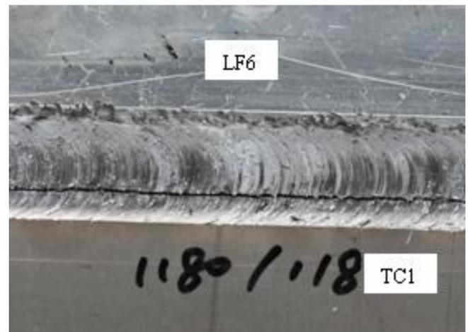
**Fig. (2).** Surface morphology of butt joint of 1180r/min.
