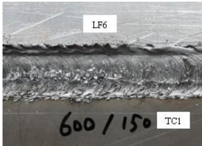
**Fig. (3).** Surface morphology of butt joint of 600r/min.
