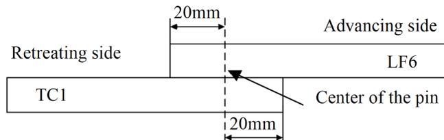
**Fig. (1).** Sketch map of relative position between Ti alloy and Al alloy of lap welding.
