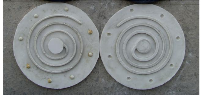
Fig. (5). Soft mold of silicone rubber.
