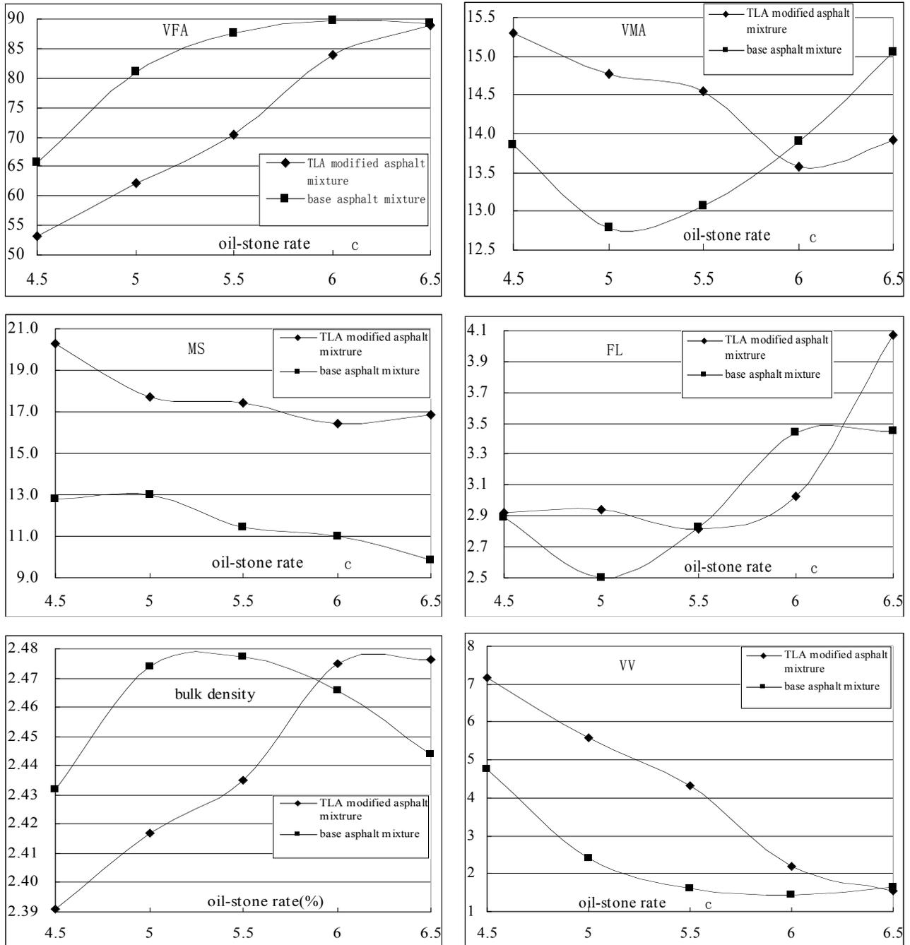
Fig. (2). The curves of physics mechanics parameter versus oil-stone rate of asphalt mixture.
