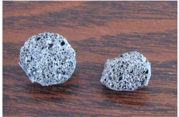
Fig. (5). Internal porous structure of ceramsite.
