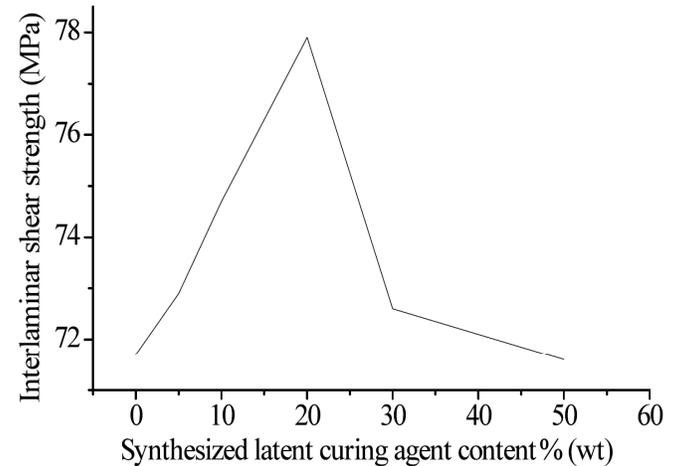
Fig. (6). Interlaminar shear strength of composites.
