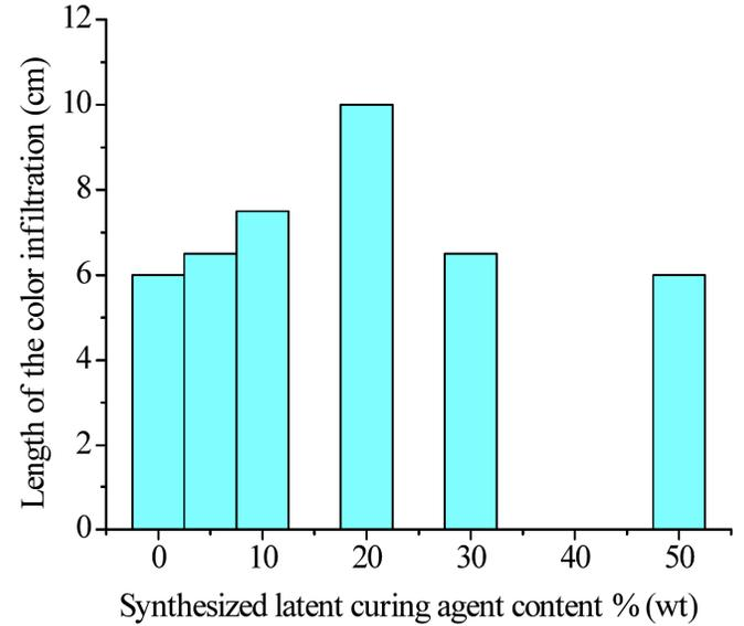
Fig. (5). Infiltrating color length of sized high modulus carbon fiber.
