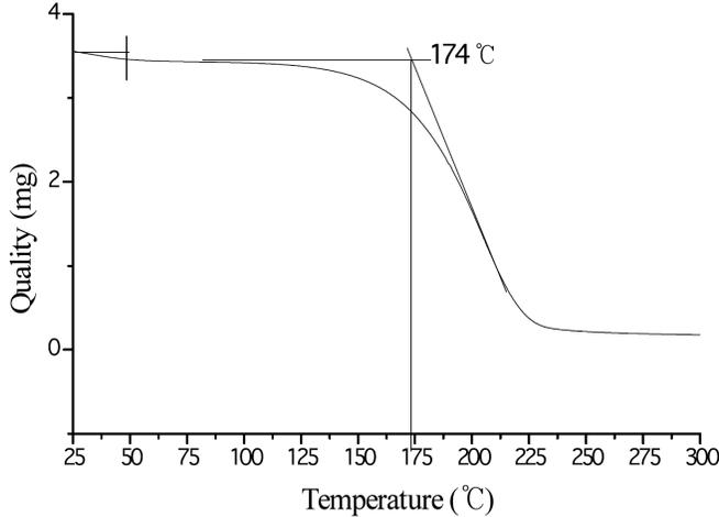
Fig. (4). TGA curve of the LCA.
