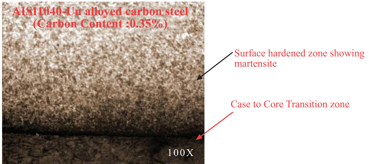
Fig. (1). Microstructure of Induction hardened AISI 1040.
