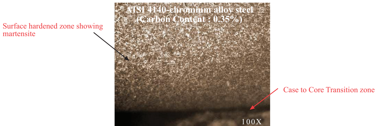
Fig. (2). Microstructure of Induction hardened AISI 4140.
