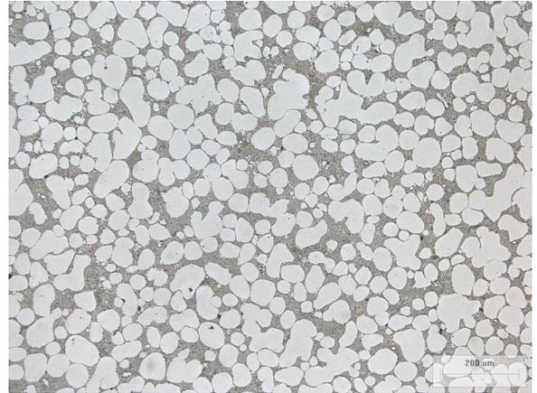
**Fig. (2).** Typical optical micrograph of SSM HPDC alloy A356 (with 0.31% Mg).
