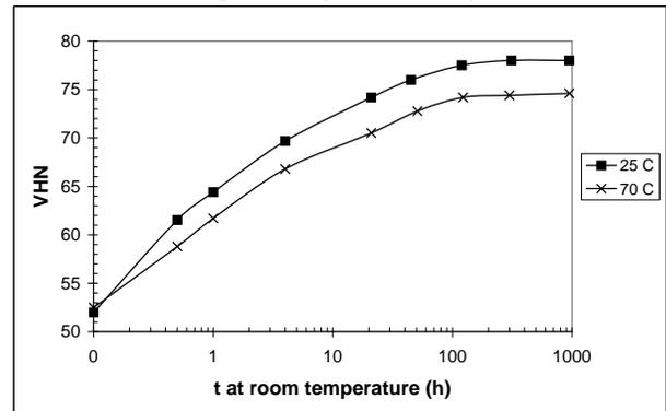
Fig. (9). Natural aging curves for 0.36wt% Mg-A356 solution treated at 540°C for 1h, followed by water quenching at 25 and 70°C.
