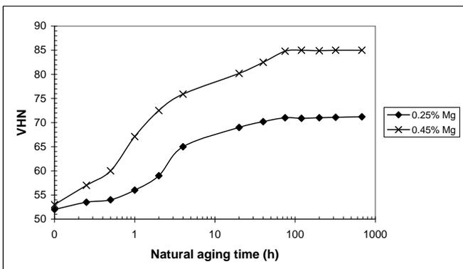
Fig. (5). Natural aging curves for SSM HPDC A356 following solution treatment at 540°C for 1 h and a water quench.
