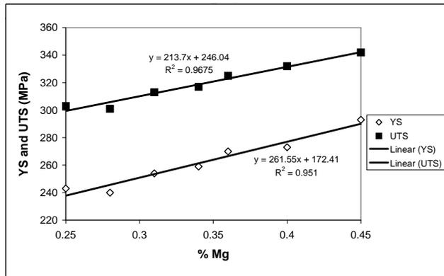
Fig. (15). YS and UTS of rheocast A356-T6 as a function of the wt% Mg of the alloy. Heat treatment: Solution treated at 540°C for 1 hour, water quenched (25°C), natural aging for 20 hours, artificial aging at 180°C for 4 hours.
