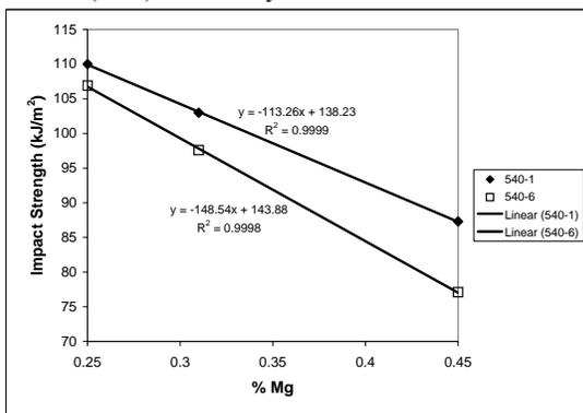
Fig. (8). Impact strength as a function of Mg-content of alloy A356-T4.
