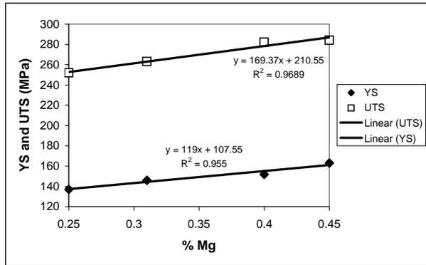
Fig. (6). Yield strength and UTS of alloy A356 as a function of the Mg-content (wt%) of the alloy for the “540-1” T4 heat treatment
