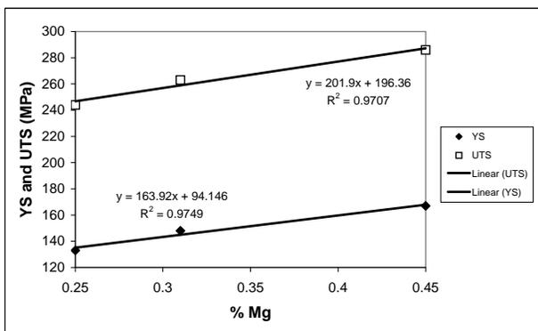
Fig. (7). Yield strength and UTS of alloy A356 as a function of the Mg-content (wt%) of the alloy for the “540-6” T4 heat treatment.
