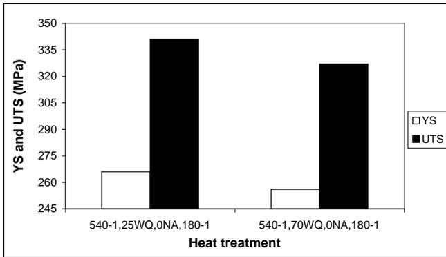
**Fig. (20).** Influence of water quench temperature on tensile properties. No natural aging prior to artificial aging at 180°C for 1 h (0.40% Mg).
