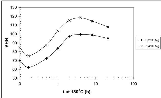
Fig. (12). Artificial aging curves at 180°C for alloy A356 (after 120 h natural aging time).
