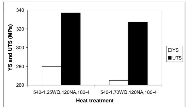
**Fig. (23).** Influence of water quench temperature on tensile properties. 120 h natural aging prior to artificial aging at 180°C for 4 h (0.40% Mg).
