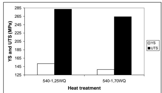
Fig. (10). A356-T4 tensile properties as a function of water quench temperature (0.40% Mg).
