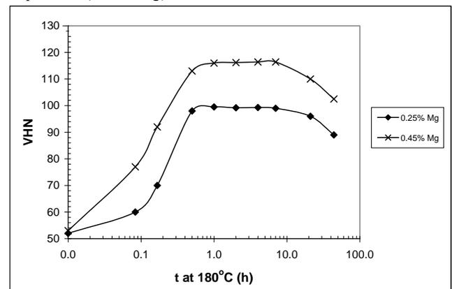
Fig. (11). Artificial aging curves at 180°C for alloy A356 (after 0 h natural aging time).
