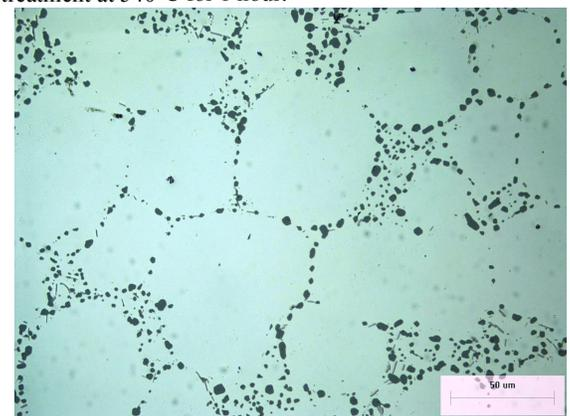
**Fig. (4).** Optical micrograph of alloy A356 (0.31% Mg) after solution treatment at 540°C for 6 hours.
