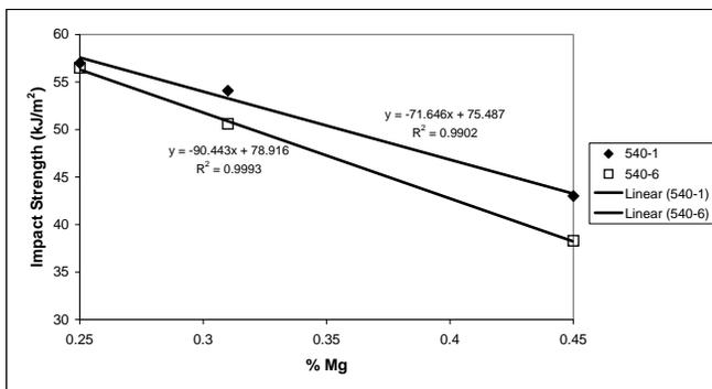
Fig. (17). Impact strength as a function of Mg-content of alloy A356-T6 (540-x,0NA,180-1).
