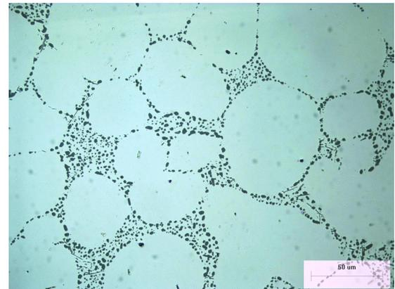
**Fig. (3).** Optical micrograph of alloy A356 (0.31% Mg) after solution treatment at 540°C for 1 hour.
