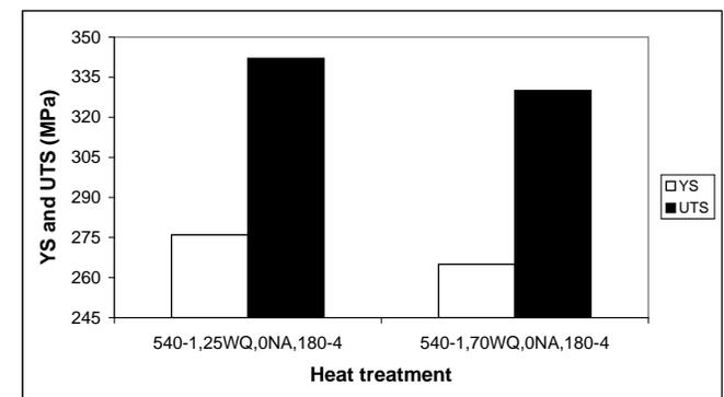
Fig. (19). Influence of water quench temperature on tensile properties. No natural aging prior to artificial aging at 180°C for 4 h (0.40% Mg).
