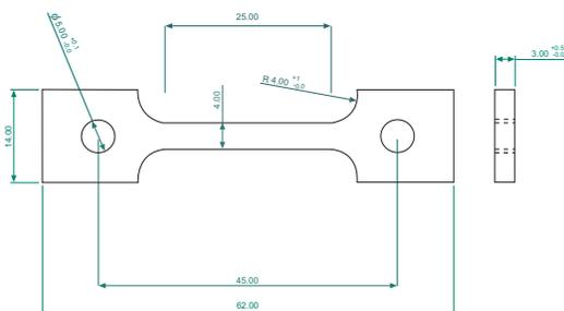
**Fig. (1).** The dimensions of the samples (in millimeters) used for tensile testing.
