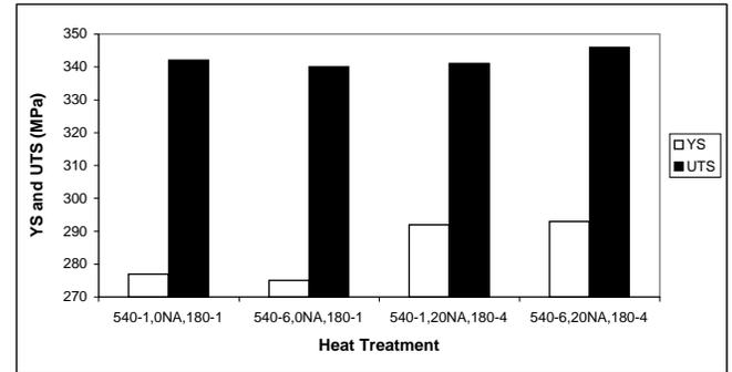
Fig. (13). Yield strength (YS) and ultimate tensile strength (UTS) of alloy A356 (0.45% Mg) as a function of heat treatment conditions.
