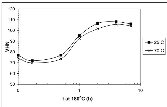
**Fig. (22).** Artificial aging curves at 180°C - water quench temperatures of 25 and 70°C were used and 120 h natural aging prior to artificial aging (0.36% Mg).
