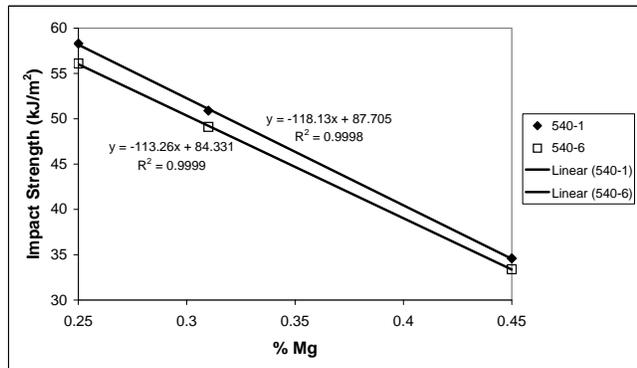
Fig. (16). Impact strength as a function of Mg-content of alloy A356-T6 (540-x,20NA,180-4).
