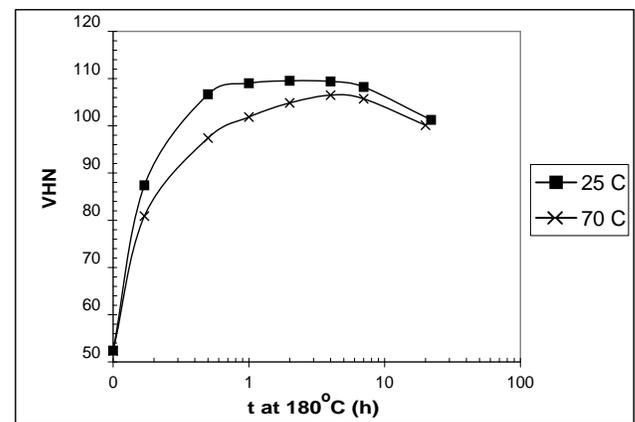
Fig. (18). Artificial aging curves at 180°C - water quench temperatures of 25 and 70°C were used and no natural aging prior to artificial aging (0.36% Mg).
