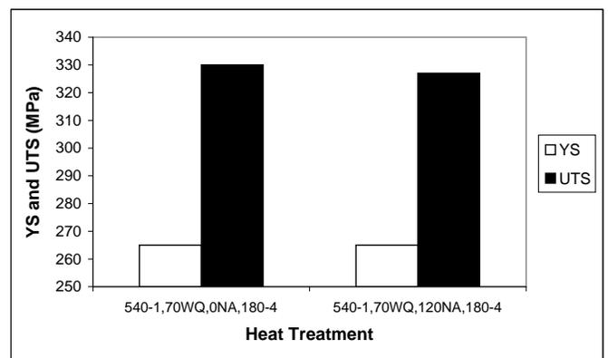
**Fig. (24).** Tensile properties for samples artificially aged at 180°C for 4 h after different natural aging periods (0.40 wt% Mg). Samples quenched in 70°C water.
