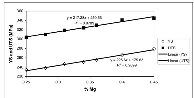
Fig. (14). YS and UTS of rheocast A356-T6 as a function of the wt% Mg of the alloy. Heat treatment: Solution treated at 540°C for 1 hour, water quenched (25°C), no natural aging, artificial aging at 180°C for 1 hour.
