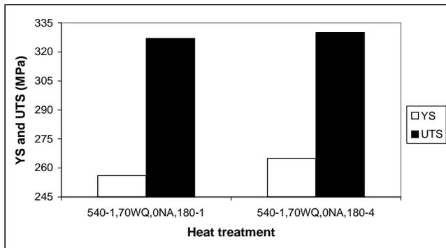
**Fig. (21).** Influence of artificial aging time on tensile properties of samples quenched in 70°C water. No natural aging prior to artificial aging at 180°C (0.40% Mg).
